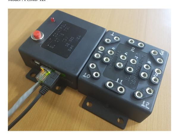
The PCMD-12P is a interface device to link your process to GAP-OSM. It is a LAN based device which can be used to connect and collect data from 12 stations. A typical usage example is, to monitor the cycle time. Each cycle time can be recorded and a report indicating the shortest cycle time, average cycle time, number of stoppages and the time duration of each stoppage, number of cycles run since the last reset etc..
